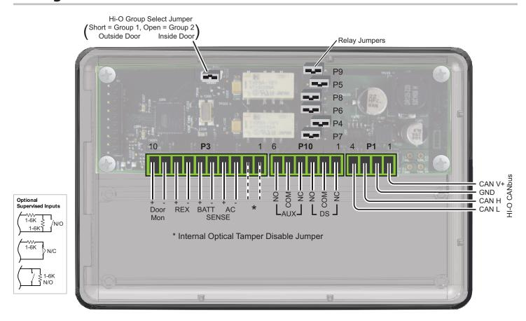
Note: Connect the Door Monitor to avoid a Force Door Alarm.
